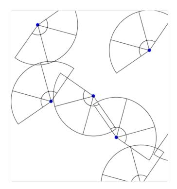
Figure 2. Pedestrian agents in the application showing the arc of their field of vision
