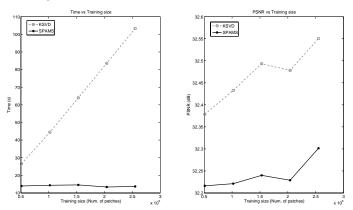
Fig. 3. SMALLbox example results - KSVD [6] versus SPAMS [10] with variable training size.
