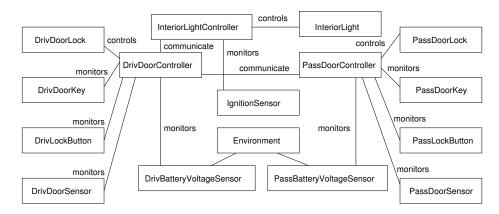
Fig. 3. Door Locking System Object Diagram
