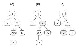
**Fig. 2.** Examples of a genetic program tree, where (a) is a tree, (b) is the same tree after a mutation, and (c) is the same tree after crossover. The shaded nodes represent the location of the change.
