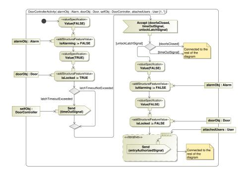
Fig. 3: Segment of the Door Controller Activity
