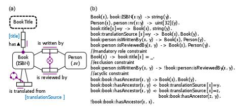
Fig. 2. (a) An ORM schema mapped to (b) Datalog<sup>LB</sup>.
