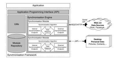
Fig. 1. Architecture of the synchronisation framework
