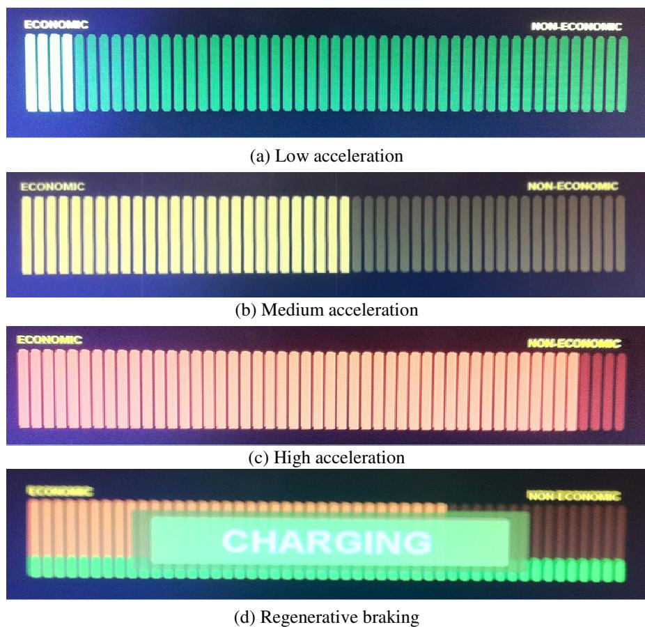
**Fig. 1.** Power-Flow Gauge Conditions
