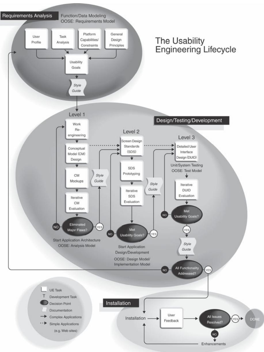
**Fig. 2.** The *Usability Engineering Lifecycle* by Deborah Mayhew. It consists of three phases – requirements analysis, development / design / testing and installation. Each phase consists of a series of tasks [12].
