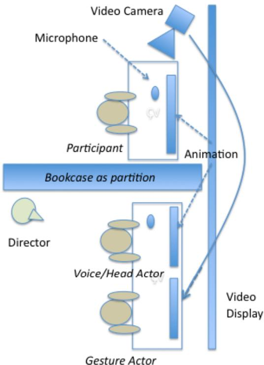
**Fig. 3.** Setup for Laboratory Tests of 3d System
