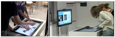
**Fig. 1.** The system includes two remotely located stations. *Right:* Participants interact on a horizontal surface while sharing the same workspace with remote partners. A vertical screen shows a video feed facilitating communication between the two locations. *Left:* Simultaneous co-located participants categorizing objects by country of origin and by functionality.
