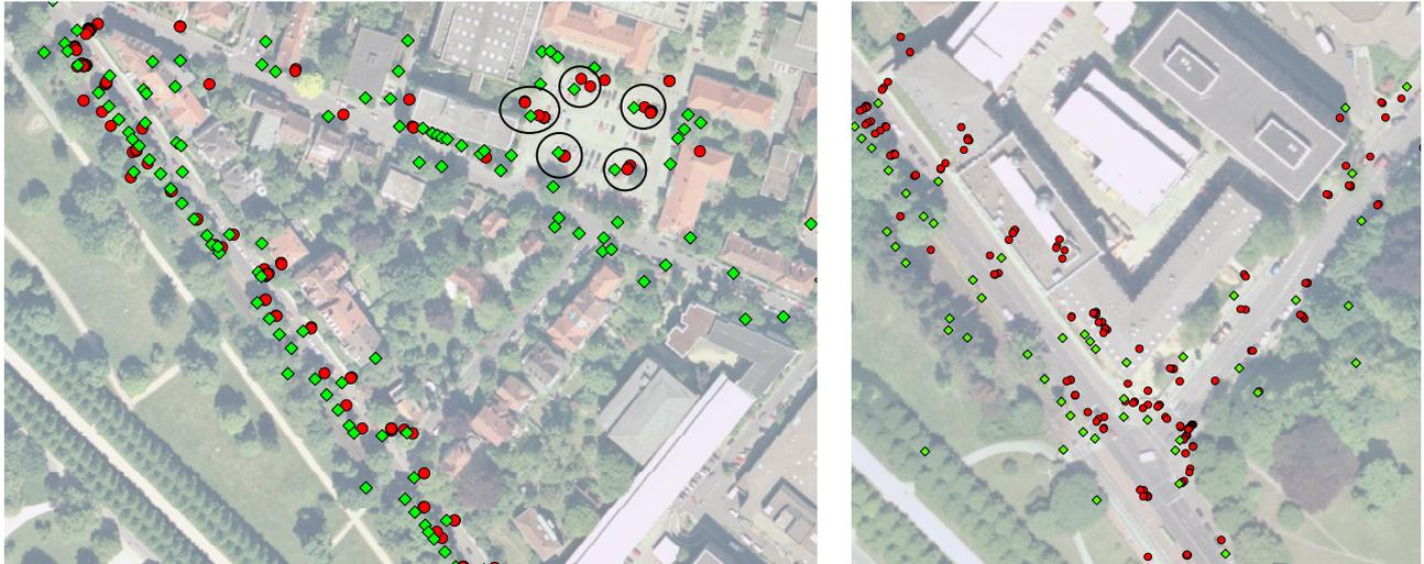
Figure 7: Comparison of reference poles (green squares) and poles extracted using the RTS Hanna vehicle (red dots).
