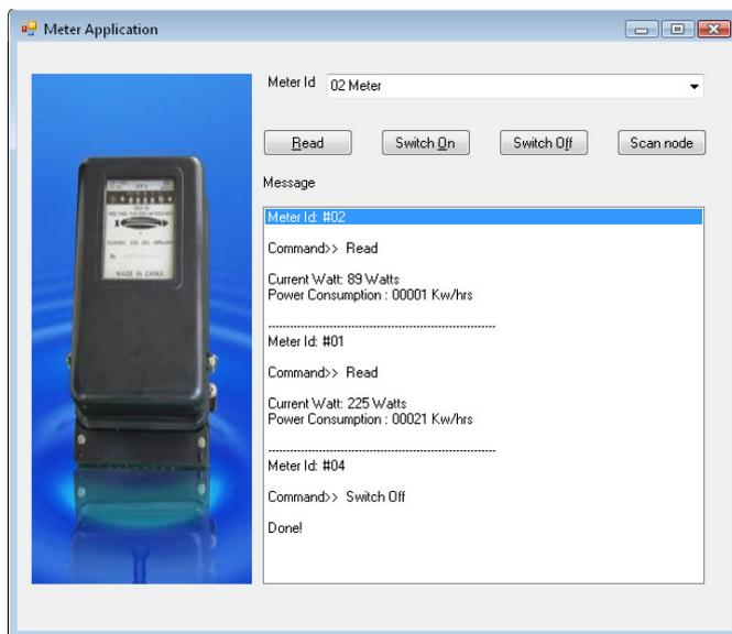
**Fig. 5** Meter application user interface prototype.
