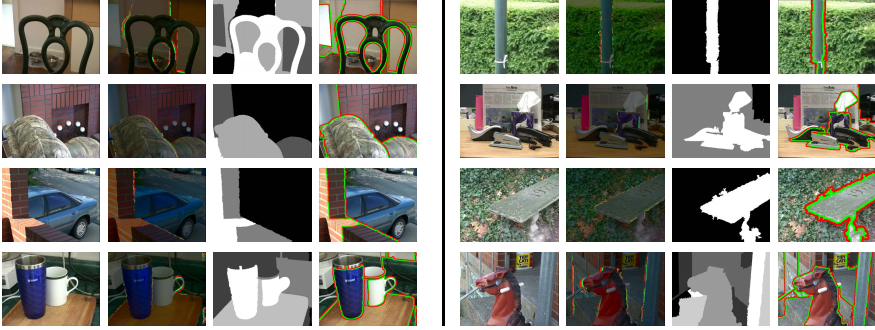
Fig. 6. Results on the CMU dataset. From left to right, for the two columns. 1) Keyframe image and 2) image with occlusion relations (green occluding, red occluded). 3) estimated depth partition, with white regions meaning closer and black meaning further. 4) Figure/ground assignment on contours with green and red overlaid marking figure and ground regions, respectively.
