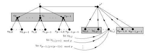
Fig. 1. The graph G(S). Edges are bought from the nodes they exit from. Notice that nodes in grey boxes are clique-connected (with arbitrary orientations), and for the sake of readability we have only inserted edges leading to node  $u_{i,j}$ .
