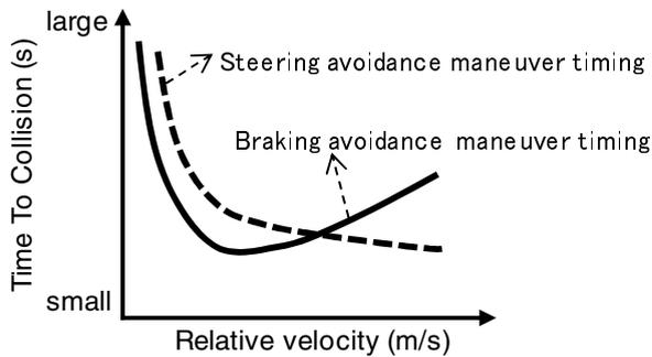
Fig. 4. Steering and braking avoidance maneuver timings
