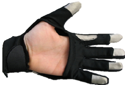
Fig. 3. MusicGlove is a sensorized glove designed to train functional hand movements
