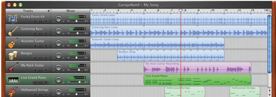
Fig. 2. GarageBand is one example of a digital audio workstation (DAW) that can interface with SMIDI instruments. Users select from a large database of instrument sounds (left) that are mapped to specific notes on the SMIDI instrument. Users can also compose music using a SMIDI instrument and a DAW (right).
