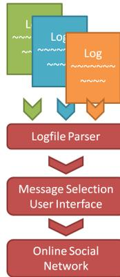
**Fig. 1.** System flowchart. Each application produces logfiles, which are then parsed to present message options to the user. The selected message is then sent to the online social networking site.
