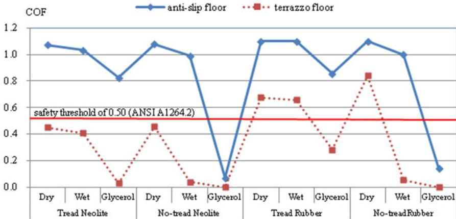
Fig. 1. The comparison of the COF under two different floors
