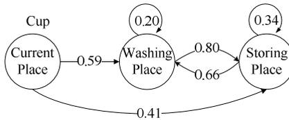
Fig. 6. Object State Machine of Object Cup
