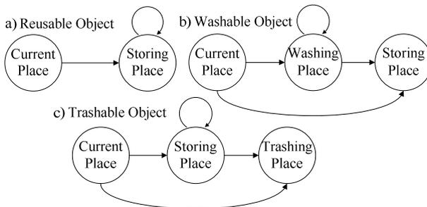
Fig. 3. State Machine of Washable Object
