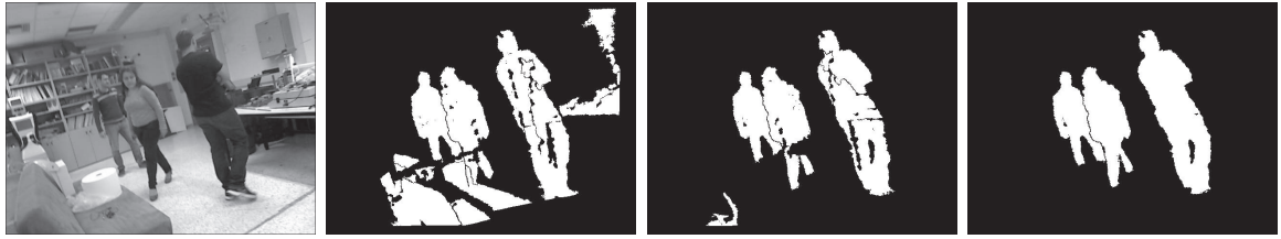
Fig. 5. Comparison of foreground detection methods. Left to right: I^0 , result using INIT, using GEN, and GEN with background history.
