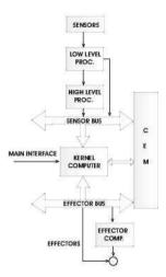
Fig. 4. Computer architecture for an integrated system
