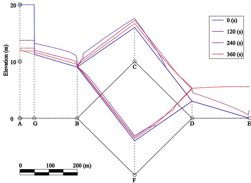
**Fig. 2.** Computed water surface profiles with the M1-scheme
