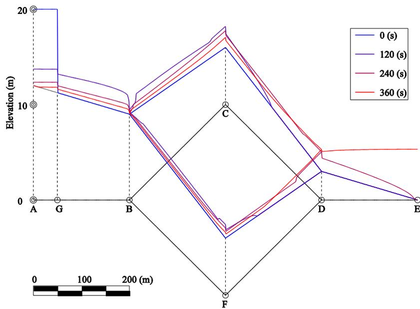
**Fig. 3.** Computed water surface profiles with the M2-scheme
