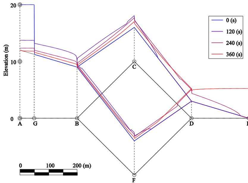
Fig. 4. Computed water surface profiles with the M3-scheme
