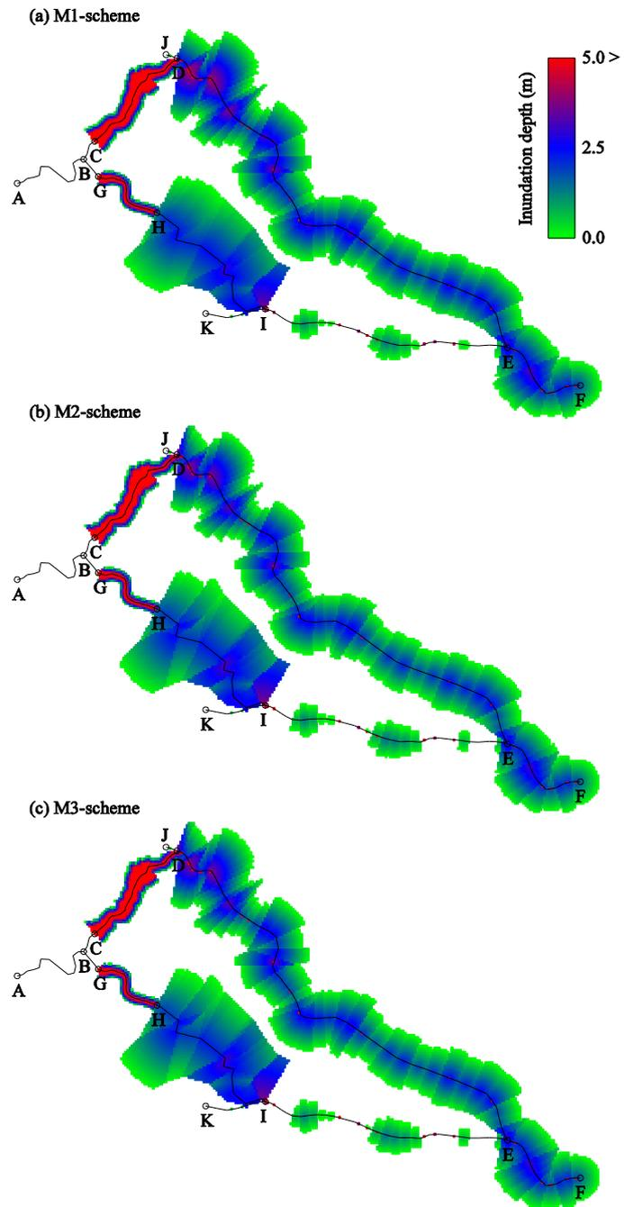
Fig. 10. Hazard maps with the three numerical schemes
