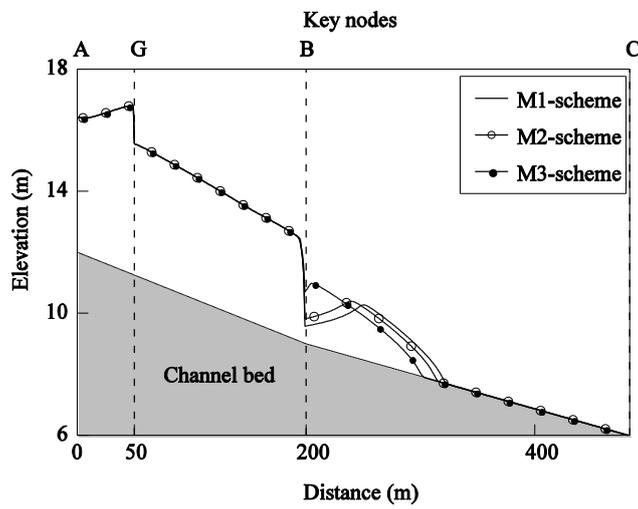
Fig. 5. Computed water surface profiles along the reaches A-G-B-C at  $t = 36$  (s)
