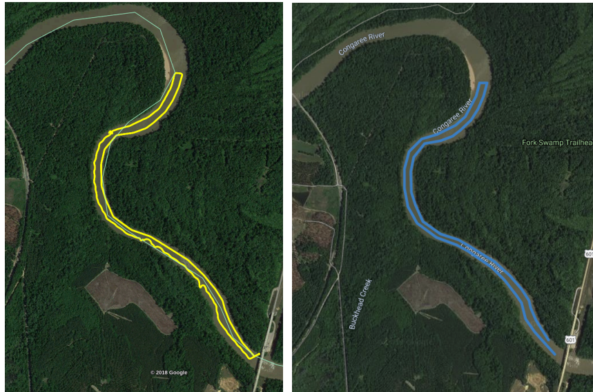
Fig. 6 The way-points for covering a river segment without taking into account meanders (right) with the actual GPS trajectory (left) executed on the 2.76km long river segment.
