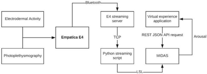
**Fig. 3** Architecture to process the physiological signals to estimate arousal levels online for interaction with the virtual reality experience. The physiological signals from the Empatica E4 wristband are transmitted to be streamed using LSL, to be analyzed online by MIDAS to infer arousal levels for a closed-loop interaction
