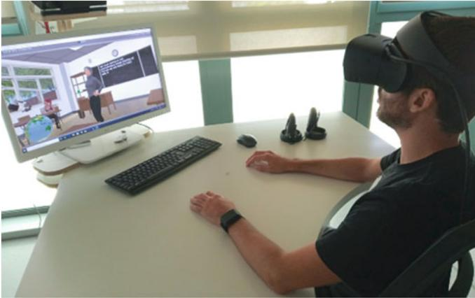
**Fig. 2** Setup of the experience. The user is wearing an Oculus Rift S headset and an Empatica E4 wristband. The computer screen allows observers to see what the user sees
