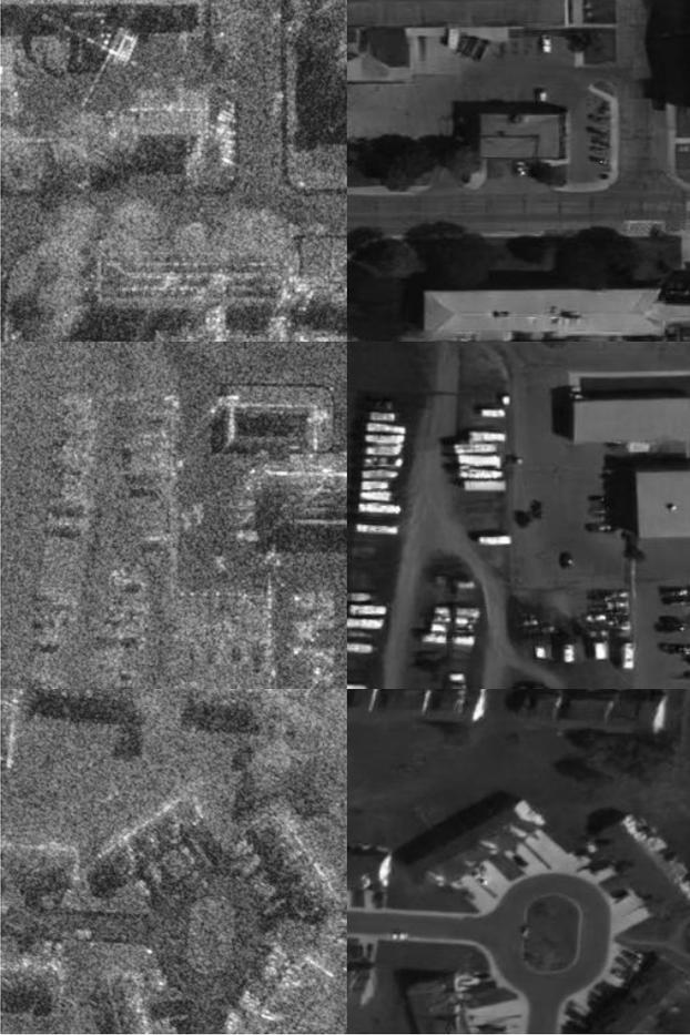
Figure 2. The examples of SAR and EO images.
