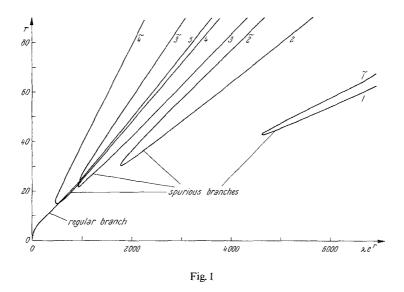
The numbers j=1,...,5 indicate the above branches. The branch 5 contains the symmetric solutions (i.e.  $u_i = u_{10-i}, i = 1,...,9$ ) which correspond to the solutions of the boundary value problem. The spurious branches with indices j=6,...,9 are related to those with j=1,...,4 by
