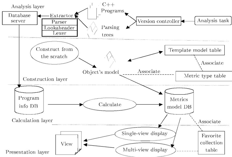
Fig.6. Layered architecture of JBOOMT.
