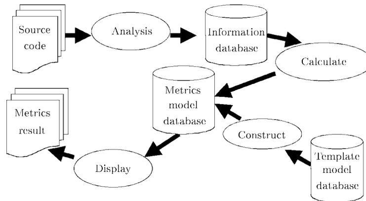
Fig.5. The workflow of JBOOMT.
