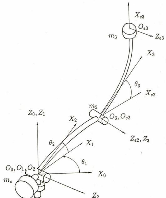
**Fig. 3** Coordinate frames of the flexible robot
