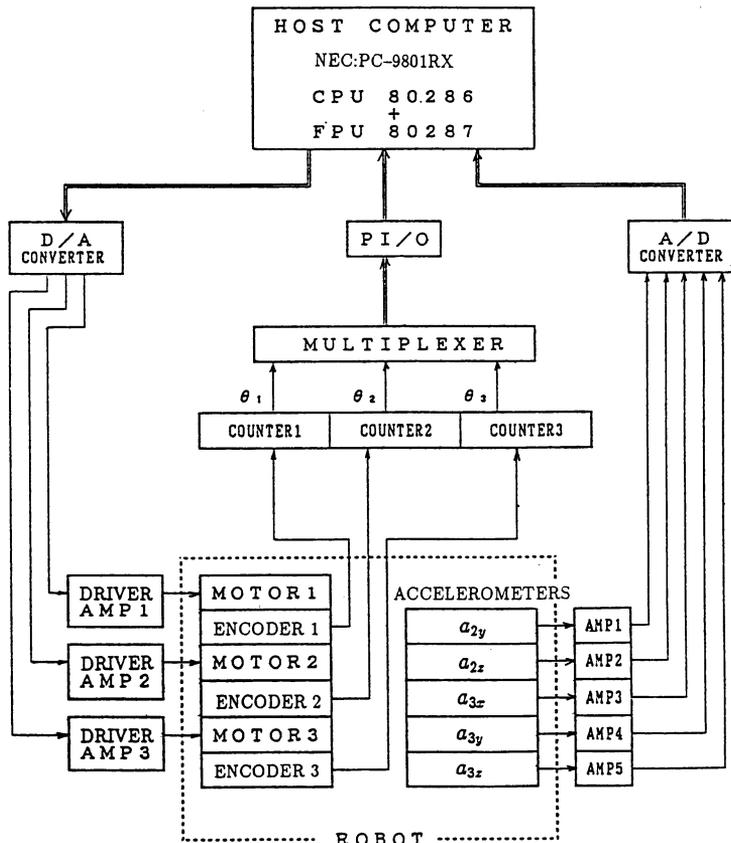
Fig. 4 Block diagram of robot control system
