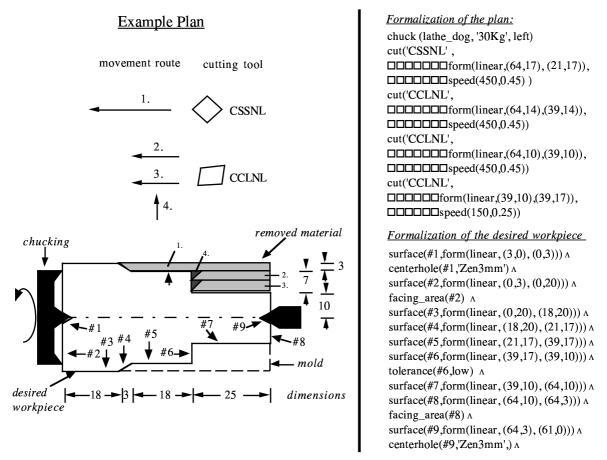
Figure 1: In this example, a mold is fixed with a lathe dog, and material is removed in four steps, in which two cutting tools with different shapes are used. The material that is removed by each step is indicated by the shaded areas on the sketch of the mold. Note that this graphical sketch is only a two-dimensional sectional drawing of the three-dimensional rotational part.
