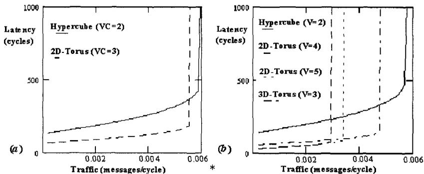
Fig. 2. The performance of the torus and hypercube ignoring the effects of wiring delays. (a)  $N=64$ , (b)  $N=1024$ .
