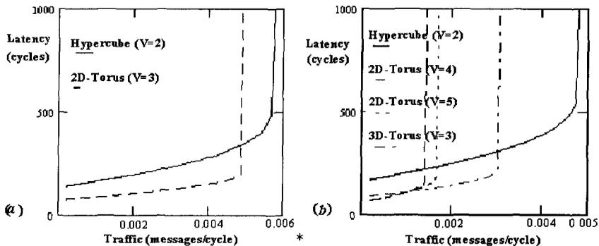
Fig. 1. The performance of the torus and hypercube including the effects of wiring delays. (a)  $N=64$ , (b)  $N=1024$ .
