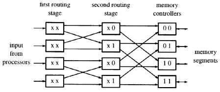
Fig. 2. Example of routing values to memory segments.
