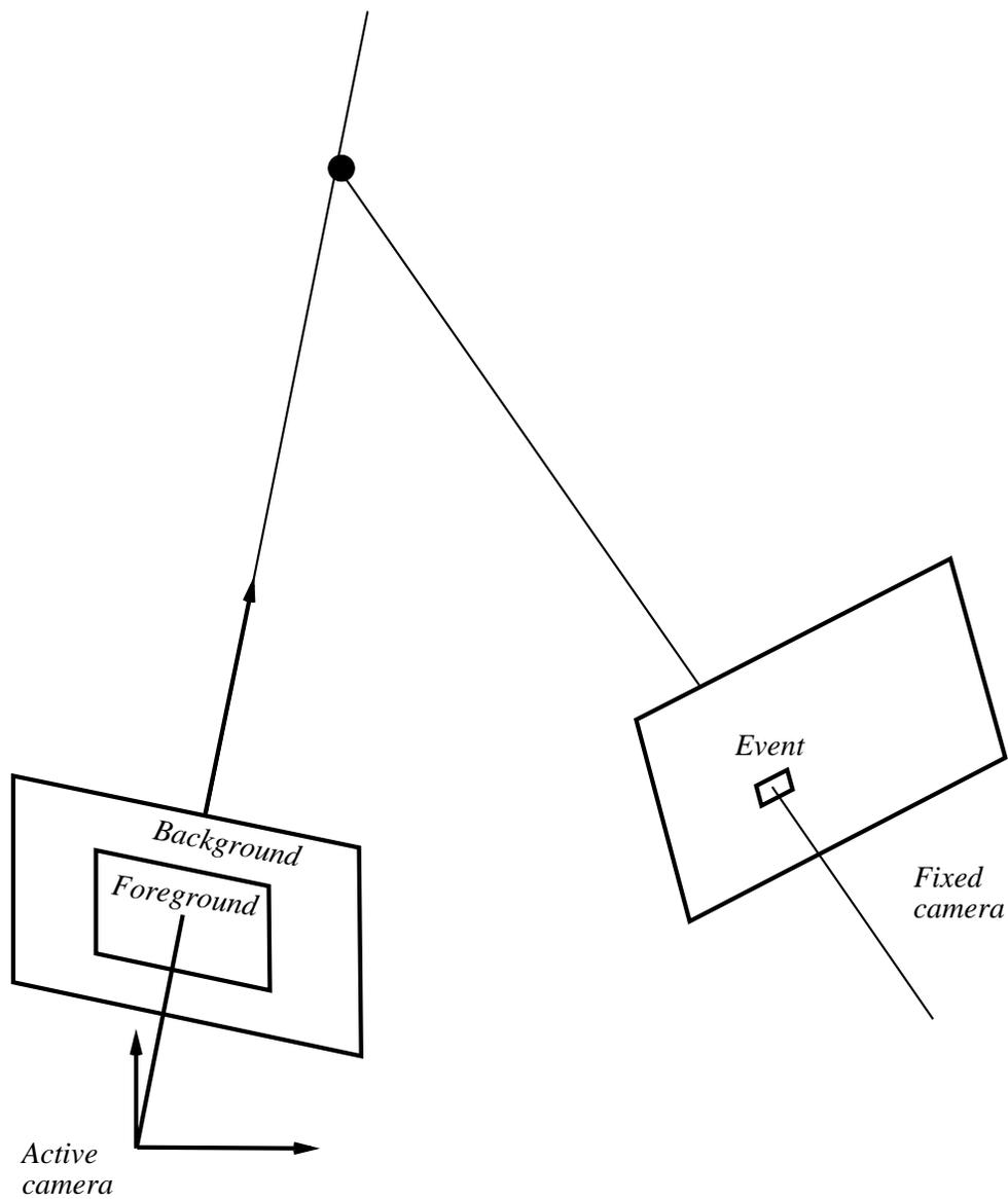
Figure 2: The coupling between the cameras allows one to associate *foreground* and *background* regions with the active camera's image. The event, which is predicted in the static camera at low resolution, must lie in the foreground region associated with the active camera's image sequence.
