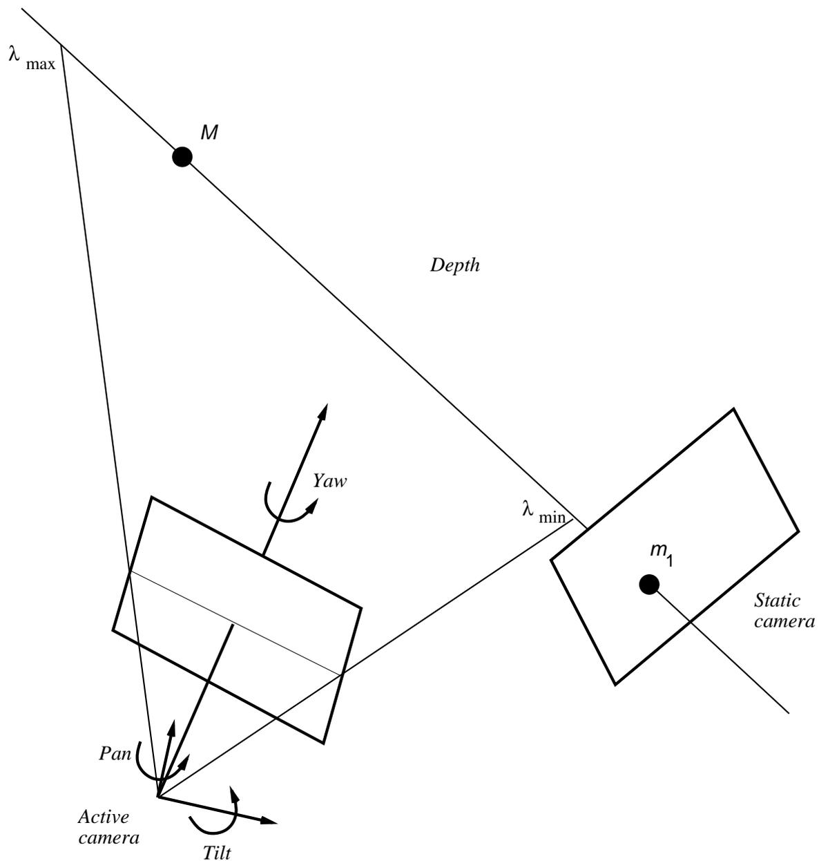
Figure 3: In order to estimate the depth to the point  $M$ , the active camera must see this point. The degrees of freedom of the active camera – pan, tilt, yaw, and focal length – are estimated such that the line of sight associated with image point  $m_1$  is seen in the active image plane.
