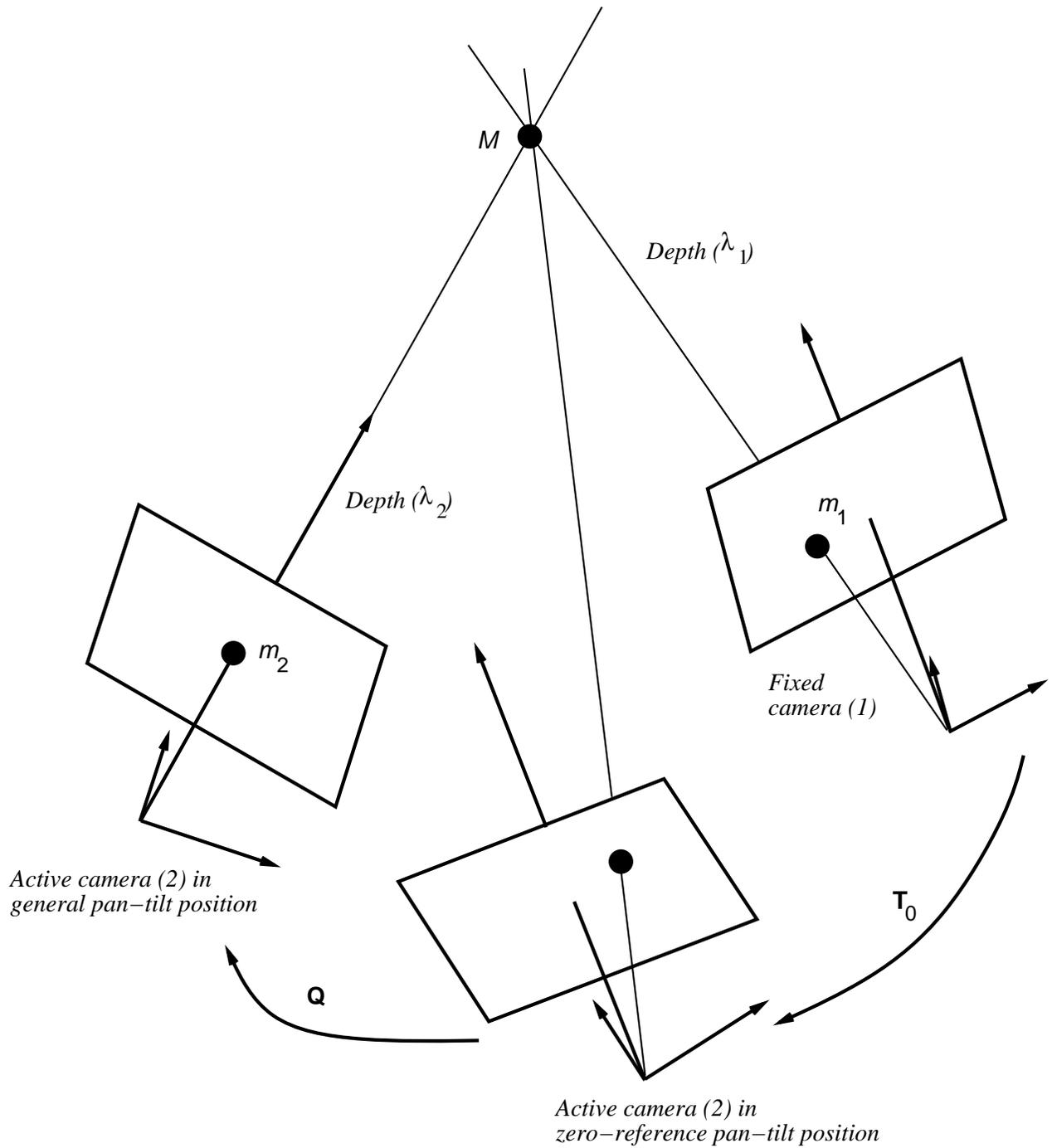
Figure 1: The active camera has a docking or a zero-reference position. Both the stereo (matrix  $\mathbf{T}_0$ ) and kinematic (matrix  $\mathbf{Q}$ ) calibrations are performed with respect to this reference position.
