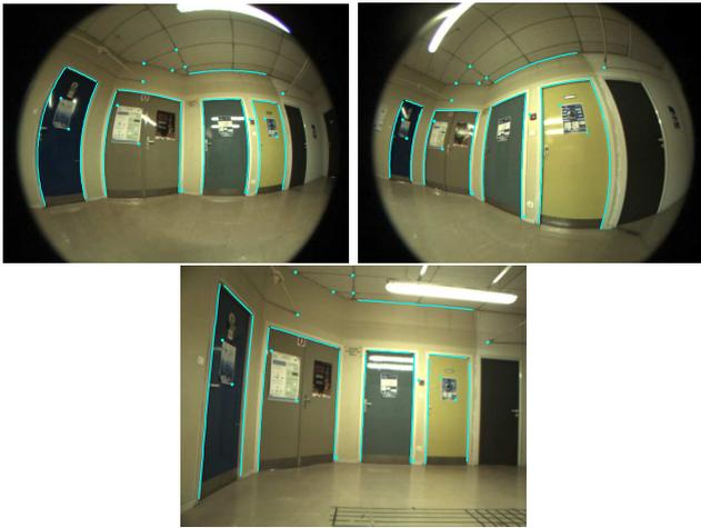
**Fig. 13** Fish-eye and perspective images with point and line correspondences
