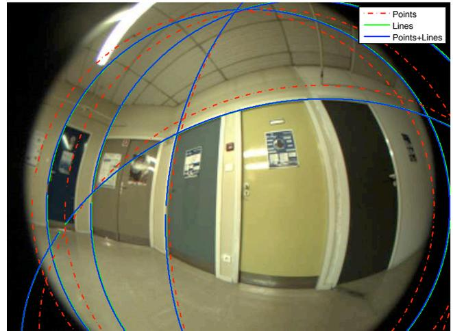
**Fig. 14** Reprojection of some reconstructed 3D lines to the first fish-eye image in figure 13. The camera poses were computed by different approaches: 5-point (red), line-based (green) and point-and-line-based (blue).
