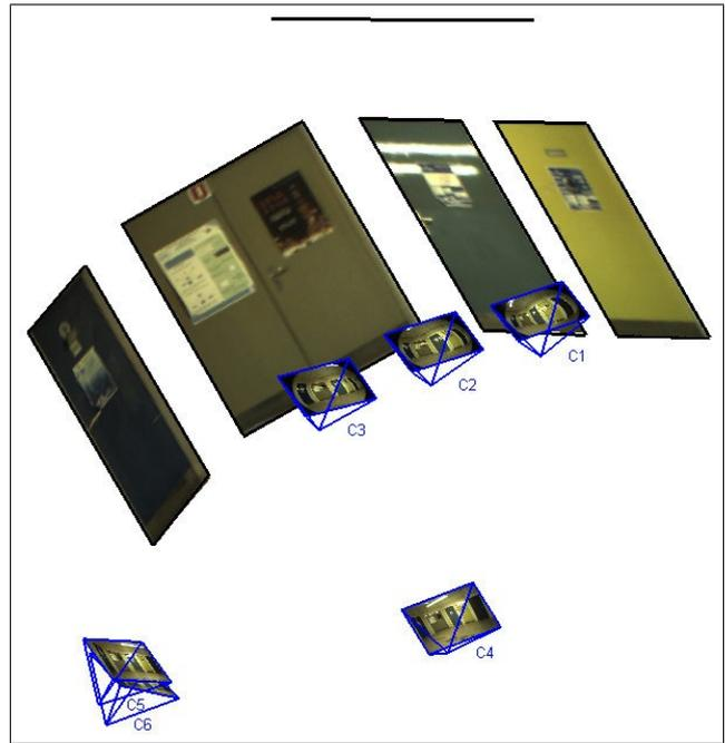
**Fig. 11** Camera poses and 3D reconstruction of the doors shown in figure 10
