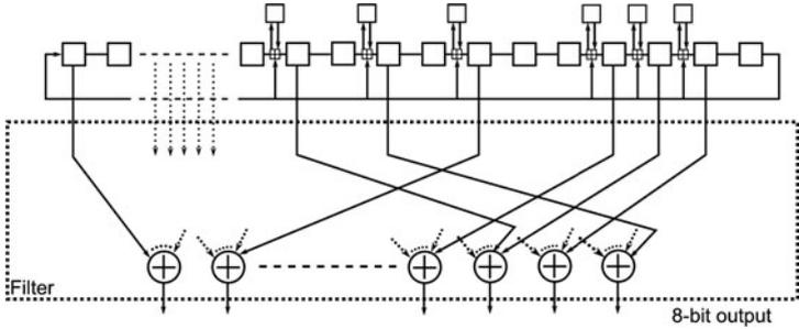
Fig. 2. An overview of F-FCSR-H and how the linear filter is used to produce the keystream.
