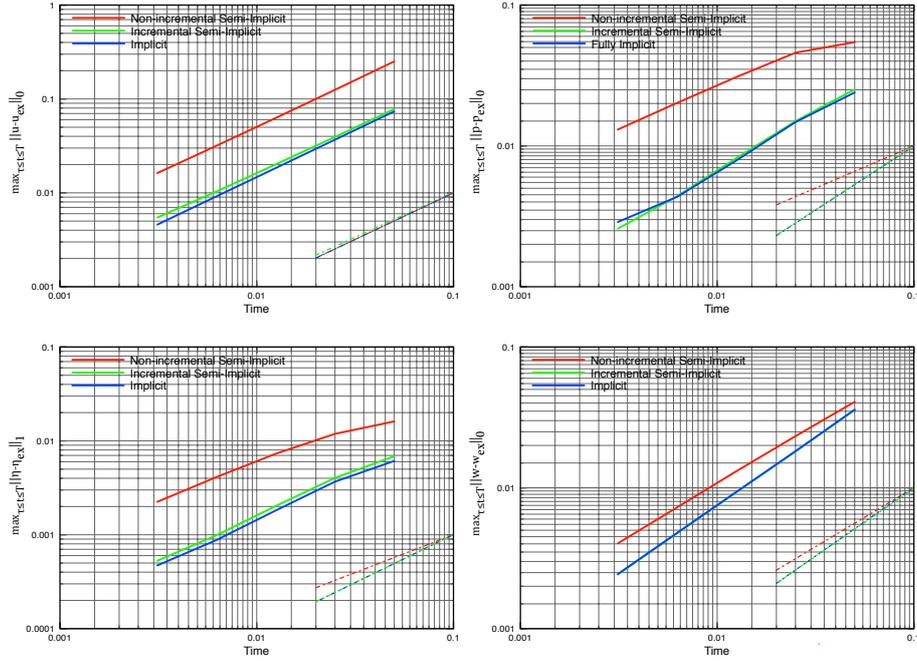
Figure 3: Convergence of the different FSI algorithms to the exact solution, for velocities, pressure and displacement. In red the non-incremental version of the semi-implicit scheme, in green the incremental one, while in blue the fully implicit scheme. Dashed lines are used to compare the slopes of the represented curves.
