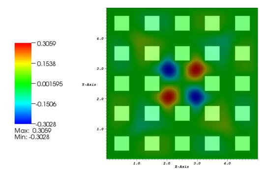
Fig. 7 A picture of the eigenfunction trapped in the defect for the TE case on a supercell with quasimomentum  $\kappa = (0,0)$  and with j = 28. The structure of the supercell is superimposed on the picture of the eigenfunction
