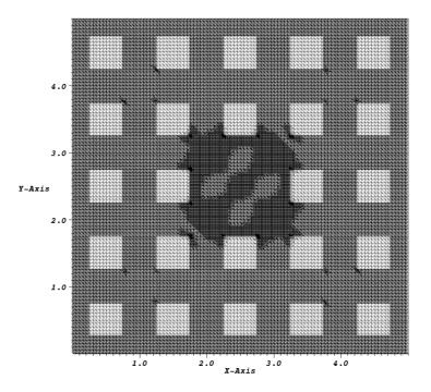
Fig. 6 An adapted mesh for a trapped eigenvalue for the TE case on a supercell with quasimomentum  $\kappa = (0,0)$  and with j = 28. The structure of the supercell is superimposed on the mesh
