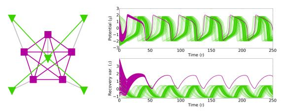
Figure 4: Synchronization of only one of two clusters in a large network of heterogeneous FN oscillators when the coupling strength takes an intermediate value. There are 100 oscillators in one cluster connected through a star graph (green) and 100 oscillators in a second cluster connected through a complete graph (magenta). The network on the left illustrates the connections between clusters (in gray) in the case of 5 oscillators in each cluster.
