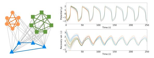
Figure 1: Cluster synchronization in a network of 17 heterogeneous FN oscillators.
