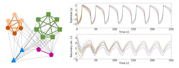
Figure 2: Emergence of new clusters, for a total of five, in the same network (as in Figure 1) of 17 FN oscillators as a result of modifying the dynamics of the two oscillators shown in magenta.
