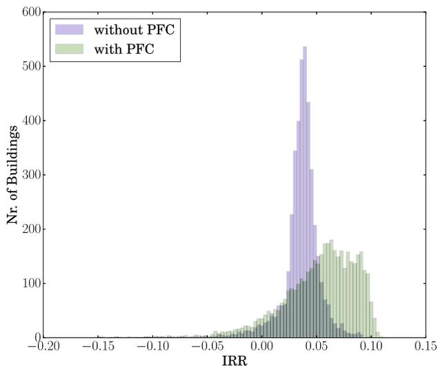
**Fig. 6** Histogram of the internal rate of return (IRR) in self-consumption mode in comparison with self-consumption mode with the provision of primary frequency control (PFC). The revenues from the PFC markets move the histogram to higher values of IRR
