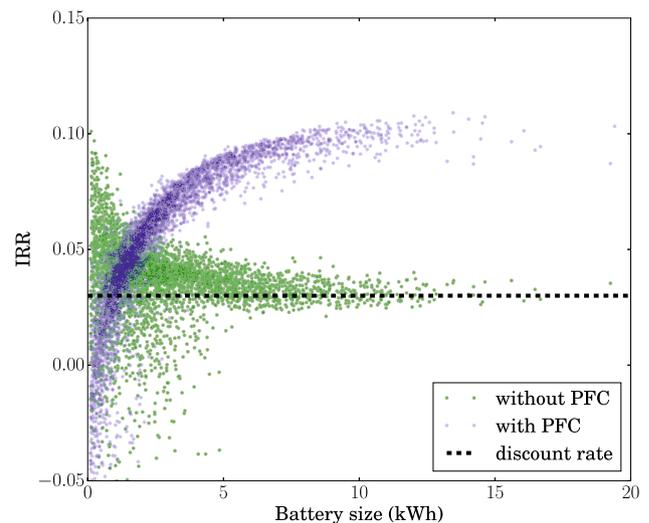
**Fig. 7** Battery size versus internal rate of return (IRR) in self-consumption only mode, in comparison with self-consumption mode with the provision of primary frequency control (PFC). Larger batteries can provide more power for PFC, which results in larger returns for larger batteries in that case
