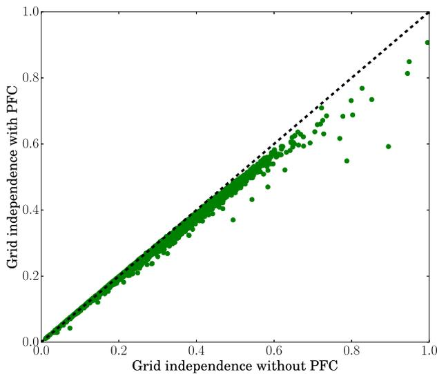
**Fig. 8** Comparison of grid independence in self-consumption mode and in self-consumption mode plus PFC. PFC provision potentially reduces the grid independence factor, because the battery is reserved for PFC in certain weeks of the year
