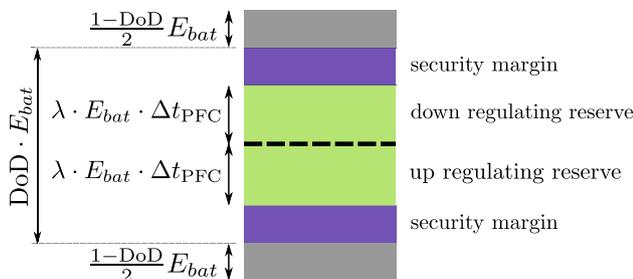
**Fig. 4** Schematic representation of reserved storage capacity for PFC. The center portion of the battery is reserved for PFC. The blue portions may be used to provide the self-consumption service. However, in this article, parallel operation of PFC and self-consumption mode is not considered. Consequently, the blue portions are assumed to represent security margins for the reserve capacity (color figure online)
