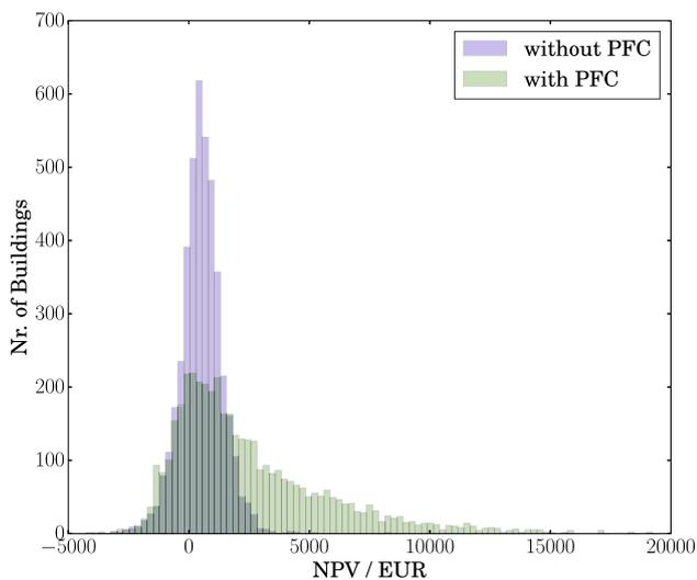
**Fig. 5** Histogram of the net present value (NPV) in self-consumption mode in comparison with self-consumption mode with the provision of primary frequency control (PFC). The revenues from the PFC markets move the histogram to higher net present values
