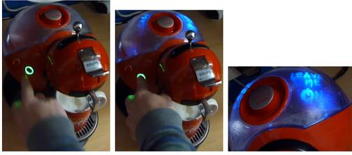
**Fig. 4** On the first image a user approaches with their finger to switch off the device. In the second and third picture, it is shown how the device informs to the intended user to not do it by activating a set of ultraviolet lights LEDs that were embedded underneath the water tank.
