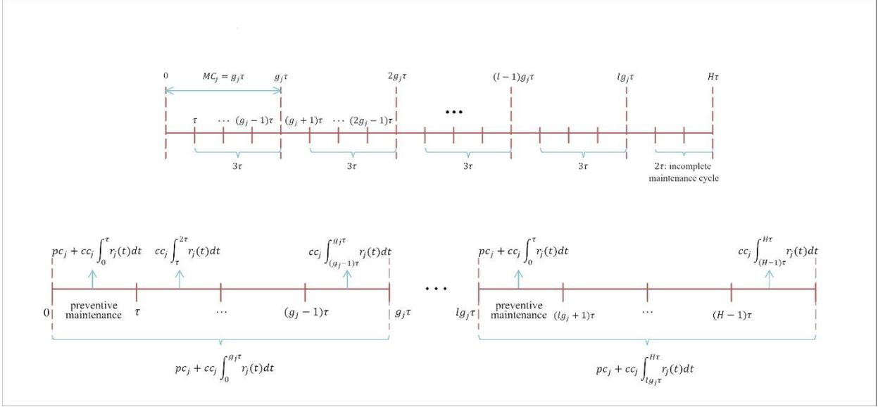
Fig. 2. The considered PM plan and cost in this study
