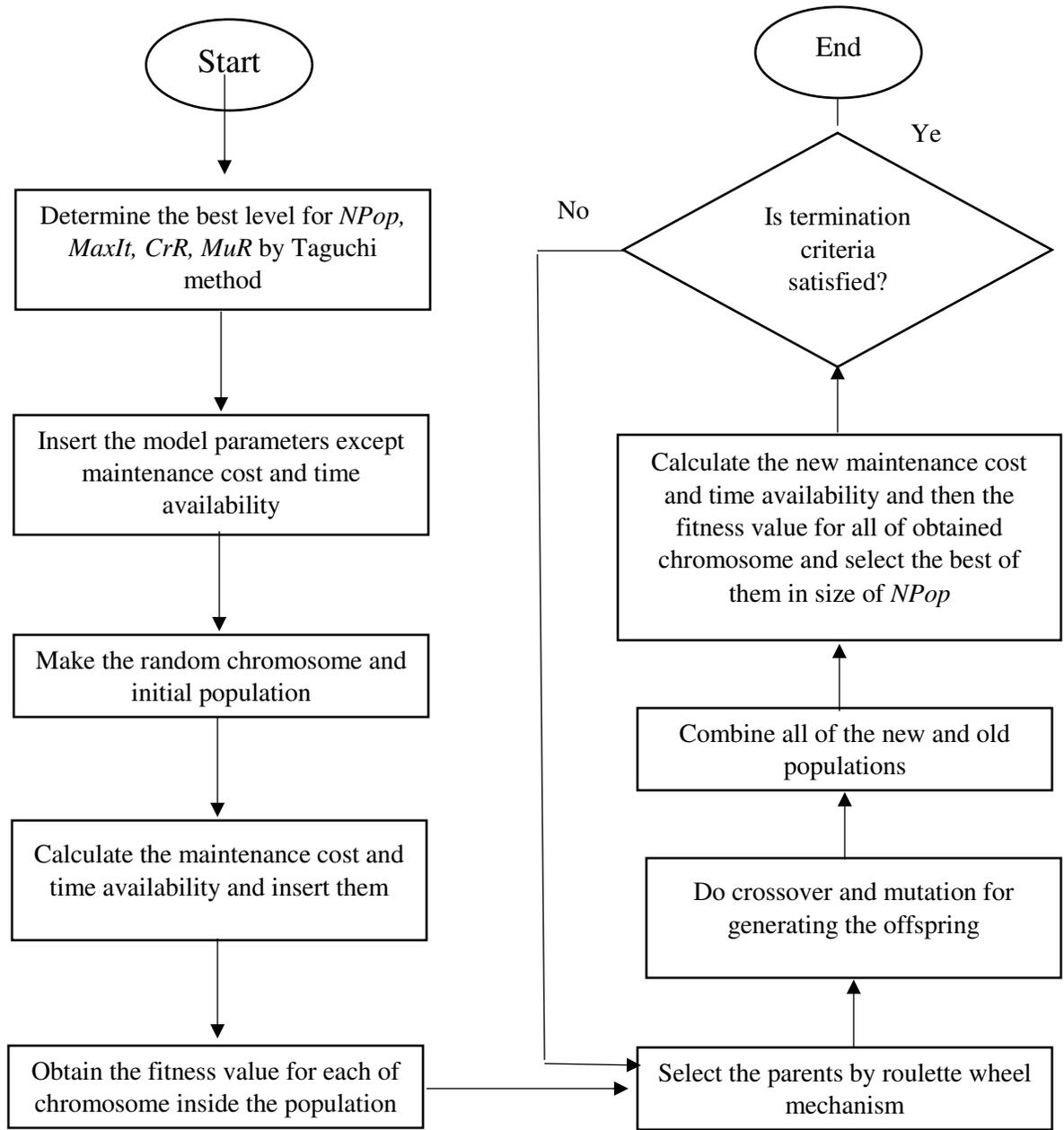
Fig. 7. The flowchart of developed GV in this study
