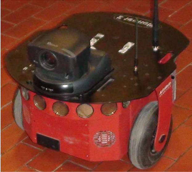
Fig. 4 Pioneer 2DX mobile robot
