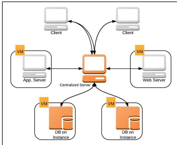
**Fig. 3: Centralized Monitoring Architecture**
