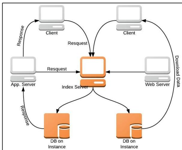
**Fig. 4: Decentralized Monitoring Architecture**
