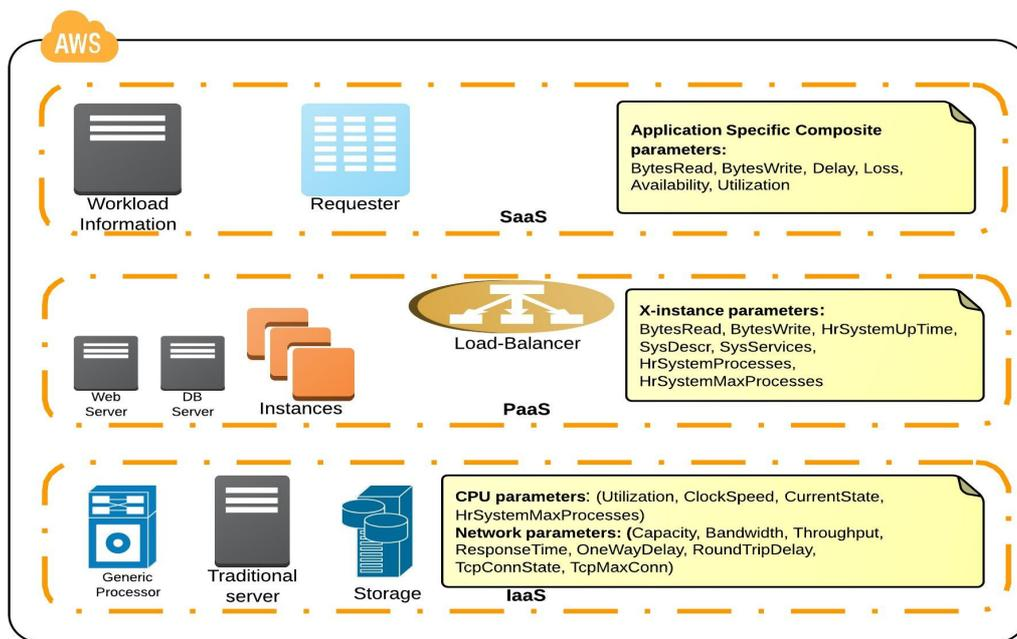
Fig. 2: Components across cloud platform layers.
