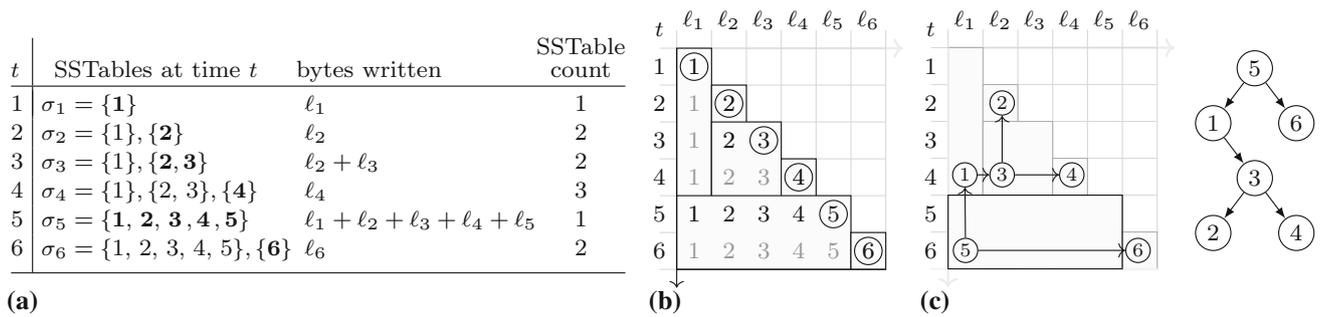
**Fig. 2** **a** An eager, stable schedule  $\sigma$  ( $n = 6, k = 3$ ). **b** A graphical representation of  $\sigma$ . Each shaded rectangle is an SSTable (over time). Row  $t$  is the stack at time  $t$ . **c** The binary-search-tree representation of  $\sigma$
