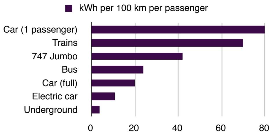
**Figure 1: Typical energy consumption of public transport. Notes: Car consuming 33mpg. Trains travelling at 33km/h, and considering energy cost for lighting, lifts, depots and workshops. 747 Jumbo at cruise speed of 900km/h. Underground average speed of 48km/h. [2]. Bus carrying 14.4 passengers at average speed of 18 km/h, distance between stops 0.3 km [3].**
