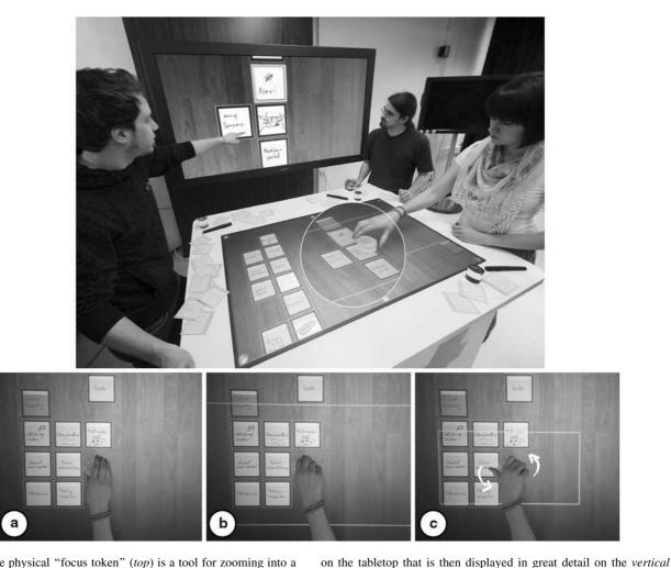
Fig. 7 The physical "focus token" (top) is a tool for zooming into a specific area of the virtual workspace. By moving and rotating the token (*bottom*, **a c**), users can move and resize a *rectangular* section
