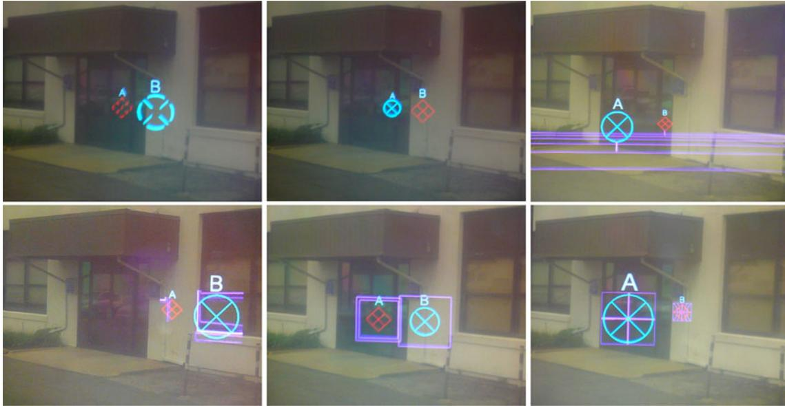
**Fig. 2** Examples of the occlusion metaphors as implemented in our user study. *Top row (left-to-right):* Stipple, Opacity, and Ground Grid. *Bottom row:* Edge Map, Tunnel, and Virtual Wall. Note that for the
