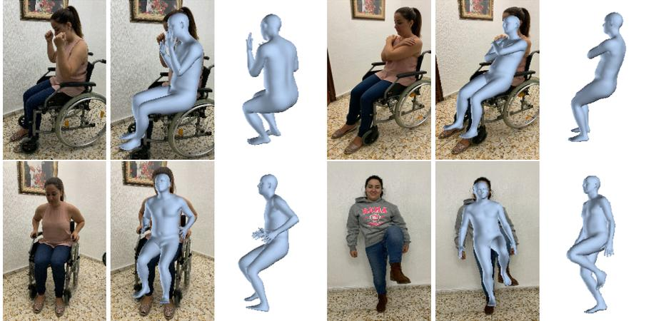
Fig. 4: . The 3D human pose estimation system is able to accurately estimate the human pose even in difficult cases such as persons in wheelchair or scenarios with high self-occlusion level caused by the exercises.
