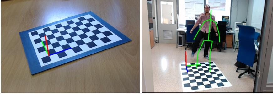
Fig. 2: A chessboard pattern is used as "the trainer's mat". It is a well-known pattern that allows the system to estimate a common 3D coordinate frame. The leftmost image depicts the pattern with the 3D axis superimposed. The rightmost image depicts the personal trainer (skeleton in green) in augmented reality in front of the patient who is imitating them. The personal trainer is rendered *in situ* thanks to the pattern's detection.
