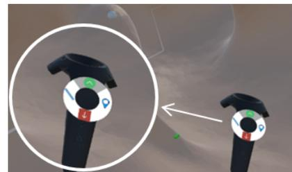
**Fig. 2** Touchpad controller indicating the direction of movement: pressing the green arrow button the user moves forward, while pressing the red arrow the user moves backwards. To tag a lesion, the user must press the marker button, confirming with the controller’s trigger button
