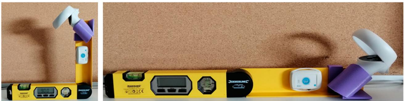
**Fig. 3** A controller holder was 3D printed, which allowed the controller to be reliably rotated by 90°. The controller could then perform three orthogonal rotations about a single axis. Both Oculus Touch v2 and the inertial sensor were attached to the digital goniometer
