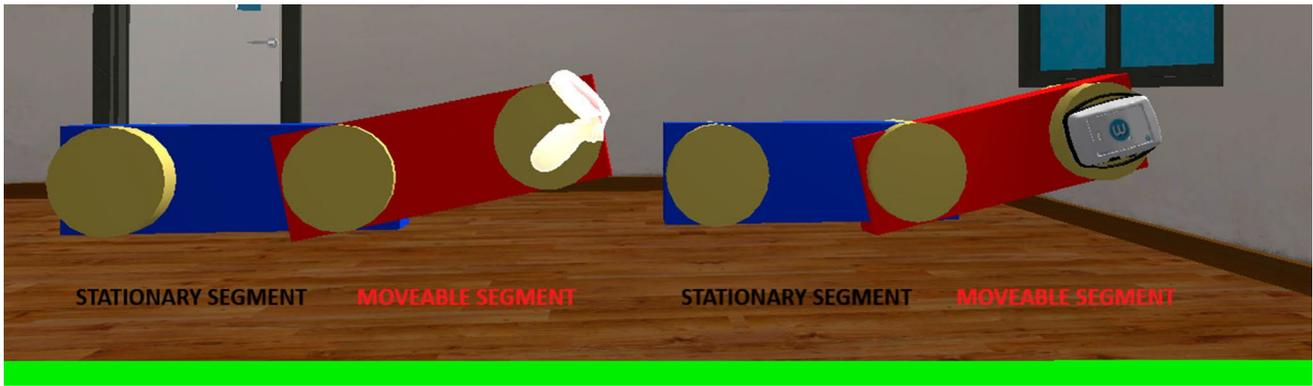
**Fig. 4** Virtual goniometers in the Unity 3D engine. The left-hand image represents the angles measured by the Oculus Touch v2 controller, while the right-hand image represents the angles recorded by the IMU sensor
