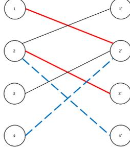
Figure 4: Graph  $\mathcal{G}_M$  corresponding to the support graph in Figure 3 (left). Bold red: Max. cardinality matching corresponding to the decomposition shown in Figure 3 (right). Dashed blue: Alternative max. cardinality matching corresponding to using edge  $(2, 4)$  twice, resulting in a length two cycle.
